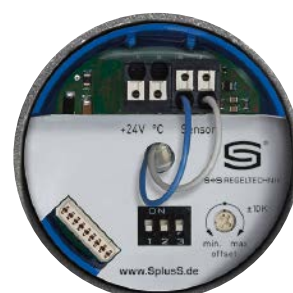
RGTM 2-I Connecting head
